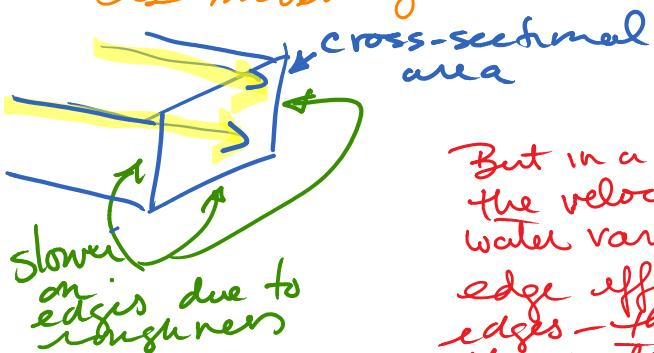
But in a cross-section the velocity of the water varies due to edge effects. Water flows slower on edges - the rougher the edge - the slower the water flows.
